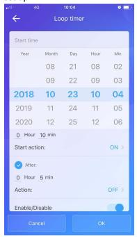
2.Take this as an example. The cycle time is set as 10 minutes, and the switch is supposed to be turned off after 5 minutes of the starting time, which is at 10:09 a.m.
